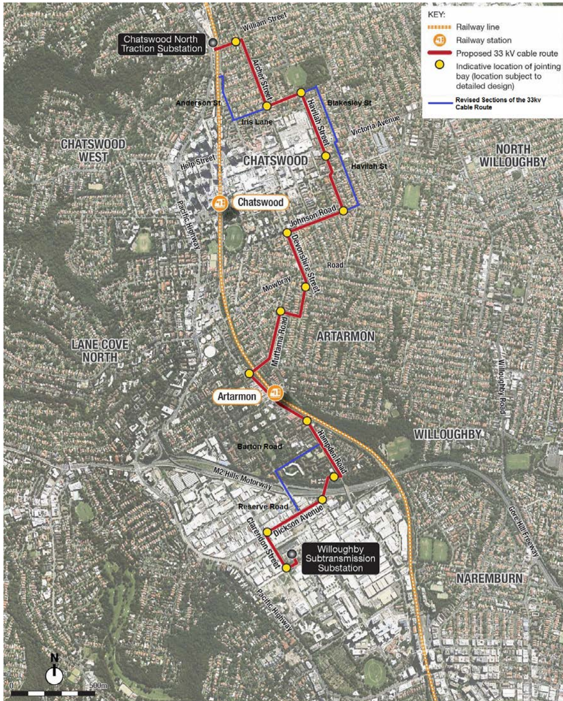
Figure 10 33kV Underground Feeder Powerline Alignment
