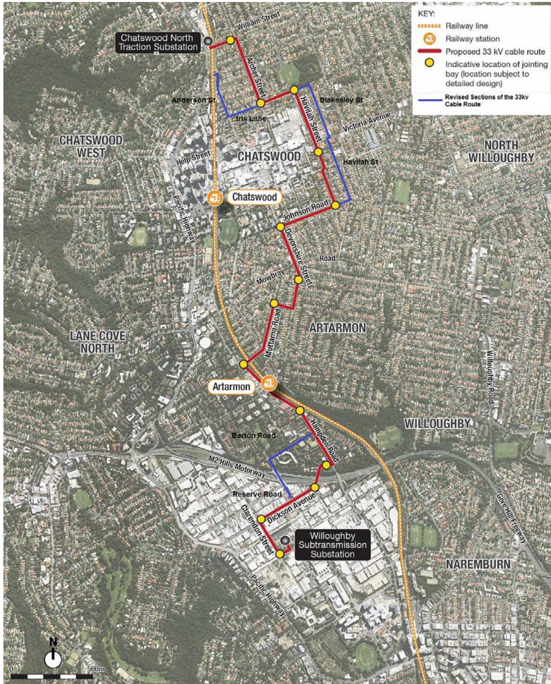
Figure 6 Overview of the 33kV Underground Feeder Powerline Route
