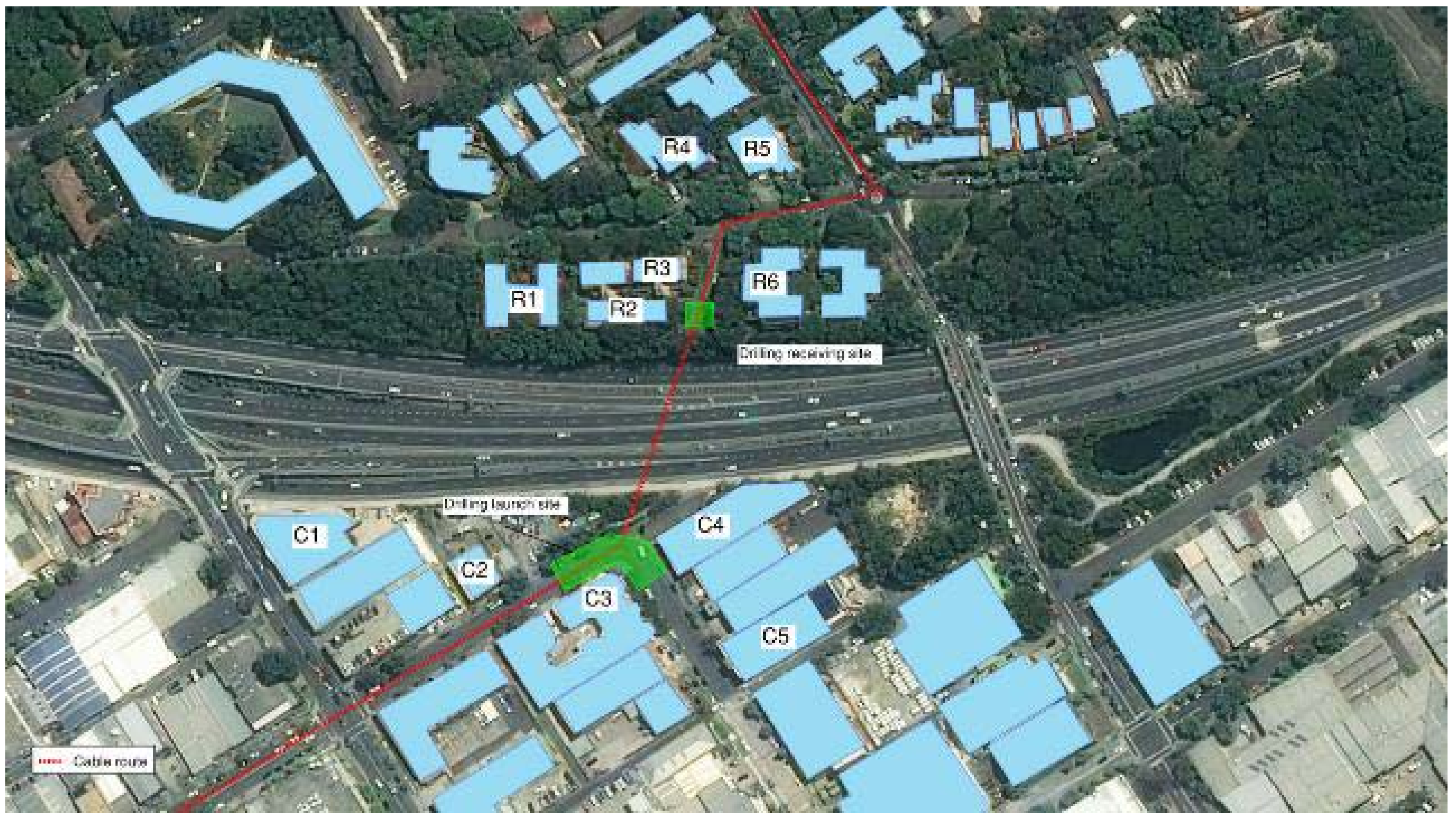
Sydney Metro Northwest – Receiver Locations for drilling under Gore Hill Freeway
